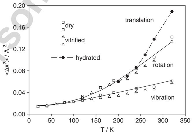
Fig. 3. Second moment of the displacement distribution at fixed time in three different environments, vacuum (dehydrated, open squares), vitrified (perdeuterated glucose glass, open triangles) and D<sub>2</sub>O-hydrated (0.35 g/g, full circles) using the thermal backscattering spectrometer IN13 at the ILL in Grenoble. The data are corrected for multiple scattering.
