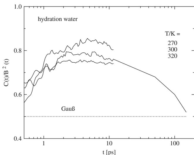
Fig. 7. Time-resolved fourth moment of the displacement distribution of protein hydration water.
